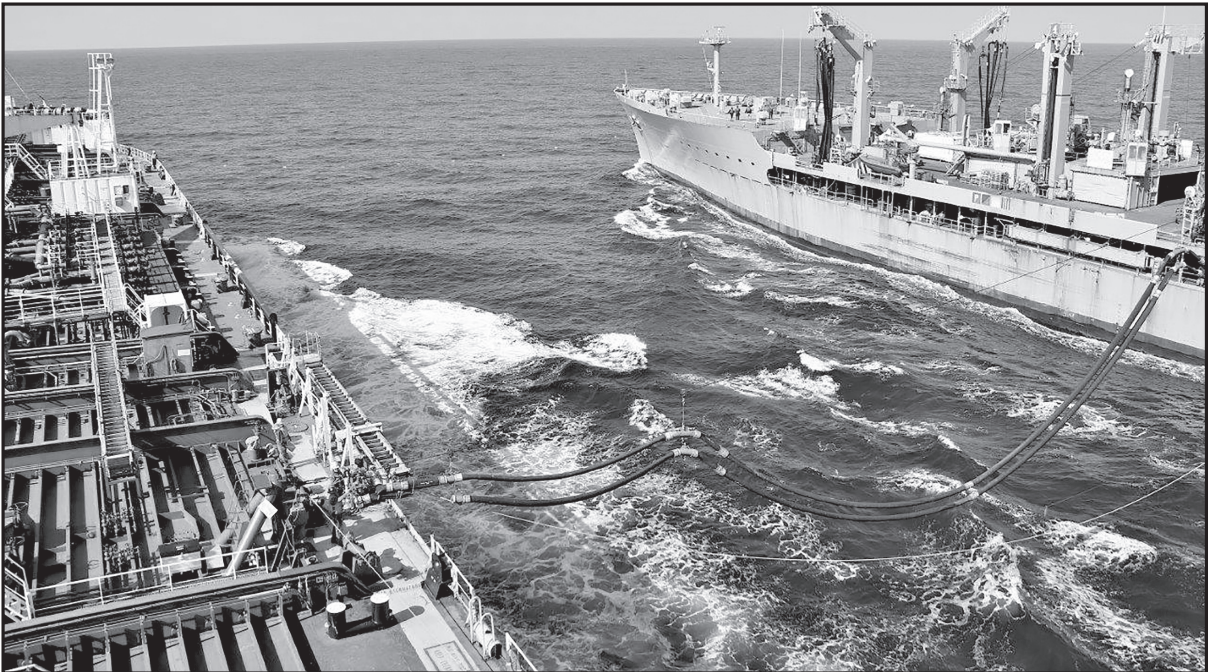
Two Seafarers-crewed vessels -- the Maersk Peary , left, and the USNS Laramie -- conduct an underway replenishment exercise near Crete.
