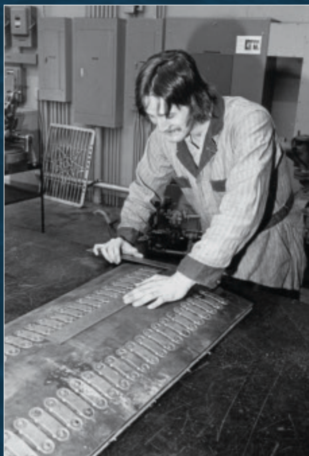
Seafarer Mike Schroble checking a belt splice as part of a 1981 Conveyor course.
