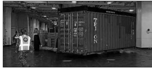
Containers are staged on the cargo decks of the USNS Bob Hope (photo above) in preparation for their eventual relocation to the vessel's main deck (photo below) where they will be loaded aboard an improved Navy lighterage for transport to designated locations on shore.
